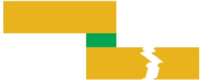
Stock break failure
