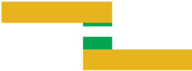
Thin Layer Cohesive failure
