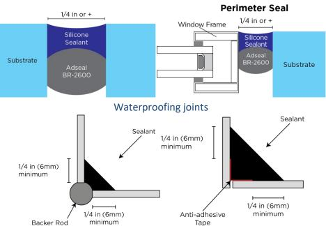
When it is not possible to use a conventional backer rod (ADSEAL BACKER ROD), it is recommended to use an anti adhesive tape.
