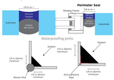
Movement joints Expansion Joint
