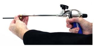
For cleaning, unscrew the extension connector, than clean the tip and the extension with the Adfoam Cleaner
