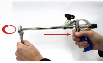
Pull the trigger to prevent damage to the needle and / or seat. Unscrew the nozzle with an adjustable wrench
