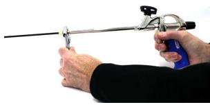
While keeping the trigger pulled, install the extension by hand and tighten with the adjustable wrench
